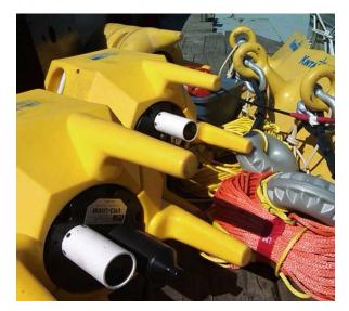
The synthetic tether used and recommended by Kintama can be made to any length and is non-corroding, positively buoyant in water, and stronger than steel (the same fiber is used for oil rig deep water mooring lines).
